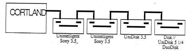
Port 5 and port 6 disk interface routines access the IWM, using slot 6 soft switches. The firmware arbitrates between slot use of the same soft switches. If a peripheral card is plugged into slot 6, the firmware in port 5 can still access the disks plugged into port 6's IWM connector by disabling the external peripheral card temporarily, performing the disk access, and then reenabling the external peripheral card.
